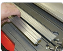
Interchangeable Splice Templates for precise pitch splicing of belts from various belt manufacturers
