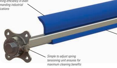
Simple snap-in-place blade design allows for easy disassembly in less than a minute — no mechanical fasteners used in the product flow and no need to remove cleaner from structure for cleaning or replacement. Reassembly is just as quick so your line is up and running again fast
