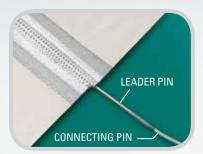
Connecting pin installation can be difficult, given both the small diameter of the pin and the flexibility of the material. To ease and speed this process we offer Leader Pins, which attach a smaller diameter, rigid lead pin to the larger diameter, flexible connecting pin. The lead pin is easily fed through the splice, allowing the actual connecting pin to be pulled through. The use of Leader Pins often reduces pin insertion time by more than 75%.
