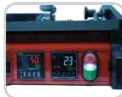
Digital Time Control with quick, simple splice settings; the Pre-Heat Setting can be used to remove moisture and avoid pinholes
