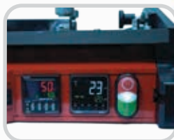
Digital Time Control with quick, simple splice settings; the Pre-Heat Setting
