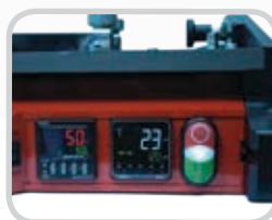
Digital Time Control with quick, simple splice settings; the Pre-Heat Setting can be used to remove moisture and avoid pinholes
