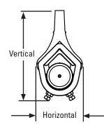
Horizontal Clearance Required Standard Duty: 4-1/4" (110 mm) Heavy Duty: 5-1/4" (135 mm)
