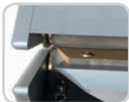
The solid fixture of the blade is guarded, with only a 10 mm (0.4") opening
