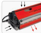
Integrated Air Cooling — cooling fans are positioned in both top and bottom beams, reducing cool down time after splice is complete. Average splice times of 8-12 minutes can be expected.
