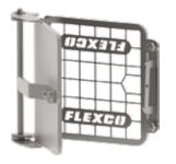
Chute Opening: 500 mm x 500 mm Outer Door: Solid c/w Lockable Handle Inner Mesh Door: 3 mm mesh @ 50 mm spacing Material: Grade 316 Stainless Steel Overall Weight: 18 kg
