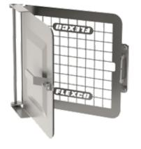
Chute Opening: 400 mm x 400 mm Outer Door: Solid c/w Lockable Handle Inner Mesh Door: 3 mm mesh @ 50 mm spacing Material: Grade 316 Stainless Steel Overall Weight: 13 kg
