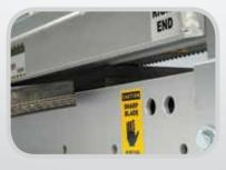
Cambered bottom beam and gently serrated grip surface provides maximum clamping force, allowing the blade to cut the belt with precise accuracy.
