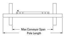
★ Each pole size can be used with a blade size either belt width minus 50mm (2"), belt width minus 200mm (8") or belt width minus 350mm (14")
