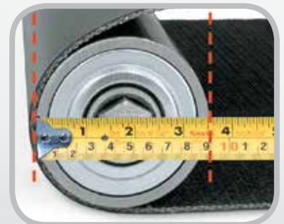
Measure smallest pulley diameter.
