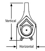
**Horizontal Clearance Required** Standard Duty: 110 mm Heavy Duty: 135 mm
