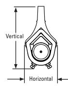
Horizontal Clearance Required Standard Duty: 4-1/4" (110 mm) Heavy Duty: 5-1/4" (135 mm)
