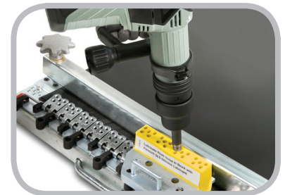
Electric Powered Rivet Driver Installation
