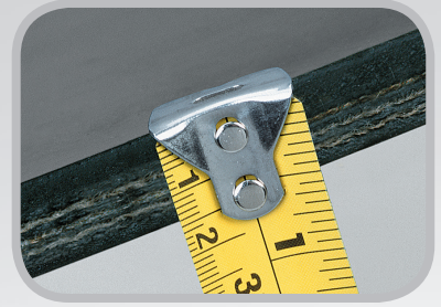
Measure belt thickness
