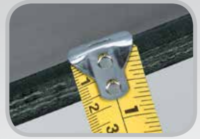
Measure belt thickness
