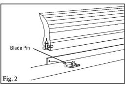
**2. Remove the worn blade.** Remove one blade pin and remove the blade from the pole (Fig. 2). Clean all fugitive material from the pole.
