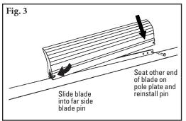
3. Install the new blade. Slide the new blade onto the pole, locking it into the far blade pin, then reinstall the removed blade pin, washer and clip (Fig. 3).
