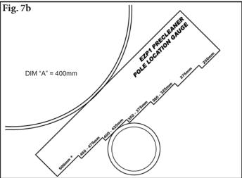
8. Confirm correct pole location. After the cleaner is installed, slide the Pole Location Gauge (provided in the instruction packet) between the cleaner pole and the pulley, until it stops at a step (Fig. 7a). Read the flat area where the pole is resting (Fig. 7b). This diameter should be equal to Dim A used in Step 1.
