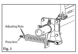
1. Remove the tension. Loosen the adjusting nuts on both sides and turn them out until they are flush with ends of the pivot arms (Fig. 1). This releases the tension of the blade on the belt.
