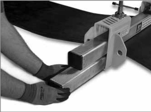
3. Slide the bottom bar into the clamp end and under the belt. Ensure the grip pattern on each bar is facing the belt surface.
