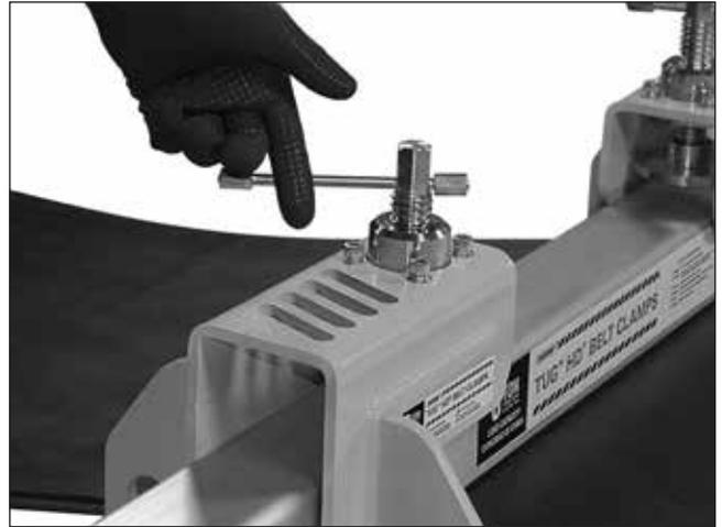
4. Use the T-handles to rapidly snug-up the clamp end. Screw against the belt. Do not hammer the T-handles to tighten the clamp ends.
