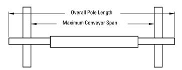
Pole Length Cleaner size + 54" (1350mm) Maximum Conveyor Span Cleaner size + 44" (1100mm)
