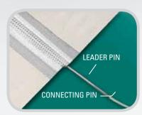
Connecting pin installation can be difficult, given both the small diameter of the pin and the flexibility of the material. To ease and speed this process we offer Leader Pins, which attach a smaller diameter, rigid lead pin to the larger diameter, flexible connecting pin. The lead pin is easily fed through the splice, allowing the actual connecting pin to be pulled through. The use of Leader Pins often reduces pin insertion time by more than 75%.
