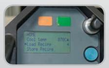
Load saved recipes to ensure consistent, high quality splice performance, regardless of which technician is operating the press.
