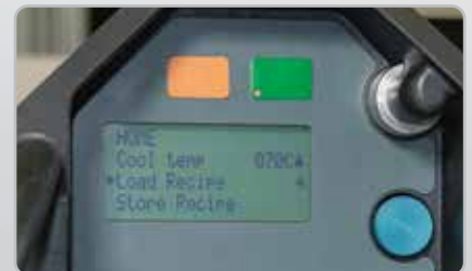
Load saved recipes to ensure consistent, high quality splice performance, regardless of which technician is operating the press.
