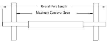
Pole Length Cleaner size +1350mm Maximum Conveyor Span Cleaner size + 1100mm
