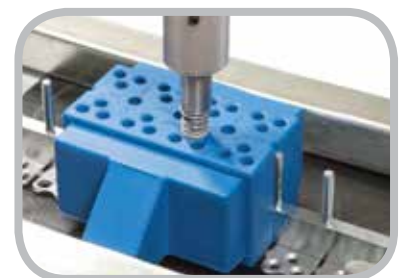
Air Powered Rivet Driver Installation
