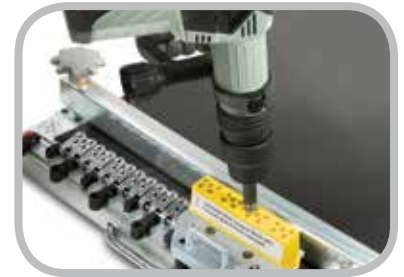
Electric Powered Rivet Driver Installation
