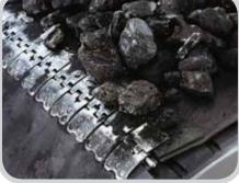
The Hydraulic Multi-Rivet Driving System delivers a strong, long-lasting splice for tough coal handling applications.
