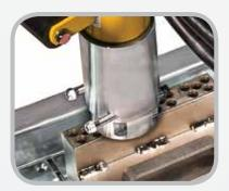
**Reduced Worker Fatigue** For faster rivet driving with less effort, simply press driver firmly into guide block and hold trigger until rivets are set.
