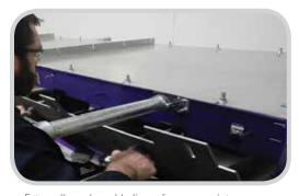
Externally replaceable liners for easy maintenance
