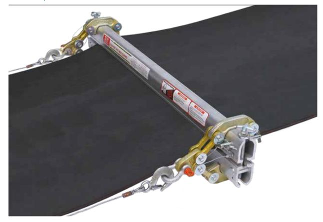
Far-Pul™ HD® clamp bars are constructed from heat-treated extruded aluminum so they resist corrosion and won't seize up in wet and corrosive environments. Clamps include adjustable steel scissors.
