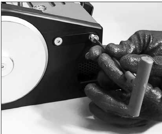
1. Loosen and remove four (4) platen locking screws.
