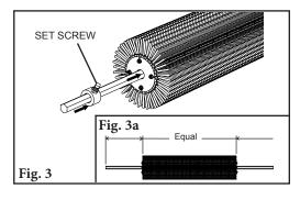
**3a. Replacing the whole drum.** Loosen the drum collar set screw and remove collar on one end (Fig. 3). Insert the drum shaft into the new drum until the drum is centred on the shaft (Fig. 3a). Replace the drum collar and tighten the set screw.
