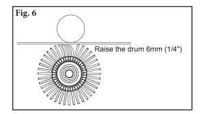
**6.** Set the cleaner tension. Once the cleaner touches the belt, raise it up 6mm with the adjustment bolts (Fig. 6). Tighten the adjusting bolt lock nuts.
