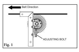
1. Remove tension from drum to belt contact. Lower the adjusting bolts to make room for the new drum (Fig.1).
