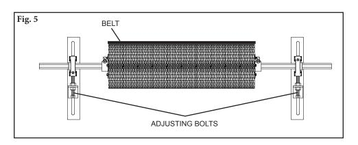
7. Set the cleaner tension. Once the cleaner touches the belt, raise it up 6mm with the adjustment bolts (Fig. 6). Tighten the adjusting bolt lock nuts.
