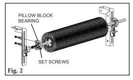
**2. Remove worn drum.** Loosen set screws on both ends. Then remove the pillow block bearing from the mounting bracket on one side. Slide the drum and shaft out of the second pillow block (Fig 2.)
