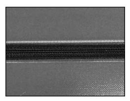
14. Fuse ASL into belt using  $Aero^{\infty}$  Press. Splice parameters will be similar as with finger splicing. Belt inner-layer should melt, flowing slightly past belt ends, but not reaching spiral loops.
