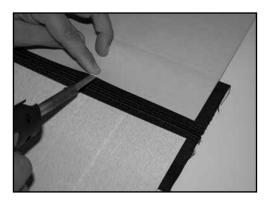
10. Using a soldering iron, fix ASL into belt at this position, fusing belt inner-layer to adhesive-primer on ASL. Belt end should follow stitch line across belt width, assuring a square splice. Sufficient fusing is required so that ASL does not disengage from belt during subsequent processing.
