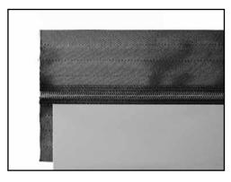
9. Insert the fabric side of the adhesive-primer coated ASL, between the separated fabric plies. ASL fabric overlap should be upwards, towards the conveying side. The ASL should extend somewhat past each side of the belt. Insertion should be to a depth where the belt ends extend to the ASL stitch line, furthest from the spiral loop.
