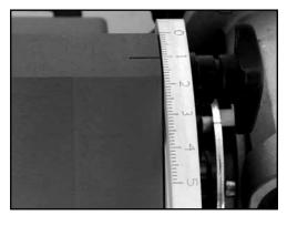
7. Using the Ply 130™, prepare belt ends. Position the Ply 130 adjustment to separate between two fabric plies of the belt. Residual of plastic inner-layer must remain on each plastic ply. Separation should be near center-plane of all fabric plies.
