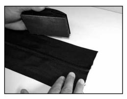
2. Using a Sanding Block / Sandpaper, lightly buff top and bottom surfaces of the fabric, raising a nap to improve mechanical bonding.
