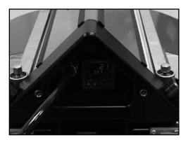
13. Place 0.5 mm silicone cloth (or silicone matrix pad) on top of prepared splice. Install Aero $^{\circ\circ}$  Press upper beam, attaching it to lower beam using connecting bolts.
