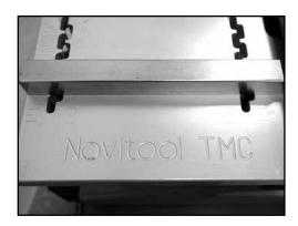
6. Using the Novitool Ply 130™ to prepare the belt ends, set the belt guide to the appropriate position as indicated in the below chart.
