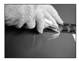
16. Remove belt from Aero $^{\infty}$  press. Use pliers to remove metal pin from ASL. Using carpenters square and knife, remove excess belt material, yielding straight belt edges.
