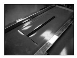
12. Place 3 mm silicone pad onto lower platen of Aero™ press. Trim ASL ends to be flush with belt edges. Place prepared ASL splice, conveying side upwards, onto 3 mm silicone pad. Fix belt in this position using Aero Belt Clamps. Fill balance of press width with belting.
