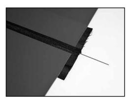
11. Insert a metal pin as a hinge pin, connecting the ASL spiral. Metal pin diameter should correspond with ASL type as indicated in the below chart. Pin should be minimally 4" (100 mm) longer than belt width.
