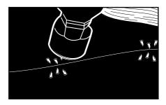
**4.** After plates are driven, cinch teeth from underside, inward toward rip. NOTE: When fastener teeth are cinched, **do not continue to hammer**—excessive hammering will weaken the repair.
