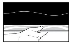
1. Place a wood support under belt where rip is to be repaired. Do not install Turtle<sup>®</sup> fasteners using the conveyor pulley or other metal surface as support, as fastener teeth would not be properly cinched.
