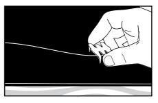
**2.** While holding ripped edges together place plates 4-6° apart with the fastener straddling both sides of the rip. A Turtle fastener may also be used at the end of a rip to prevent continued tearing.
