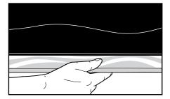
1. Place a wood support under belt where rip is to be repaired. Do not install Turtle<sup>®</sup> fasteners using the conveyor pulley or other metal surface as support, as fastener teeth would not be properly cinched.
