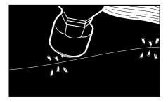
**4.** After plates are driven, cinch teeth from underside, inward toward rip. NOTE: When fastener teeth are cinched, **do not continue to hammer**—excessive hammering will weaken the repair.
