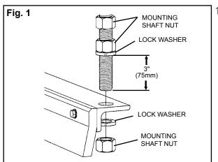
1. **Loosen mounting shaft nuts.** The bottom two mounting shafts nuts on both sides of the plow should be loosened so that the worn blade will have no tension to the belt (Fig 1.)
