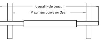
Vertical Horizontal Horizontal Clearance Required 100mm (4") Vertical Clearance Required 250mm (10")
