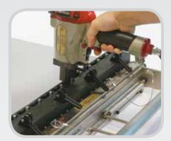
Fasteners and belt are inserted into the base where the pre-staked staples are driven through the belt with simple trigger pulls.
