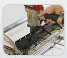
With additional trigger pulls, the staples receive their final set and the compression fit is obtained.
