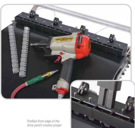
compression set of the front edge of the fastener plate.
