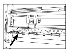
**5.** Turn tool on its side and identify the three screws that secure the anvil to be replaced.
