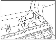
**13.** Replace guide block and cam lever. Tighten cam lever. Do not use tool for 24 hours to allow Loctite to dry.
