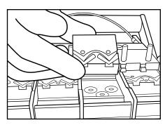
8. Remove damaged anvil from the tool.
