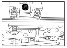
10. For tools with anti-lifting mechanism only: Replace the anti-lifting mechanisms from the top of the tool. Next, apply Loctite to the end of each screw (total of 4) and slowly thread until they have engaged in the tool. Replace the (4) springs and continue to tighten the screws (screws go through the center of each spring) until fully seated.
