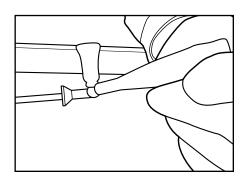
**9.** Open enclosed Loctite tube and apply Loctite to the three anvil screws included in this package.
