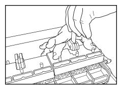
**1.** Release cam lever, press down block and turn cam lever counterclockwise.
