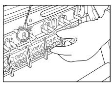
**11.** Hold anvil plate, line up screws, and tighten all three screws.
