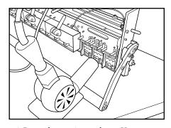
**6.** Put on heat resistant gloves. Use a 1500W heat gun on high and heat the anvil for approximately 10 minutes. (Caution - Please read all manufacturer instructions on proper use of the heat gun). This will loosen the Loctite. Allow time for plate and screws to cool.
