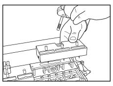
**2.** Lift cam lever and remove cam lever and guide block over the damaged anvil.
