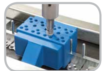
Air Powered Rivet Driver Installation
