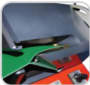
Separate between the plies
