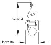
**Horizontal Clearance Required** 114mm (4-1/2") **Vertical Clearance Required** 279mm (11") (Single Cartridge) 318mm (12-1/2") (Dual Cartridge)
