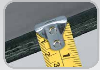
Measure belt thickness
