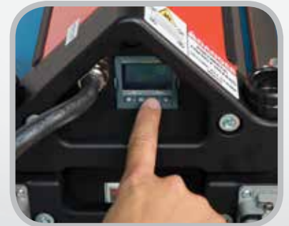
Setting temperature and pressure controller
