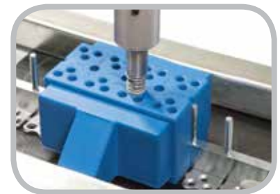
Air Powered Rivet Driver Installation
