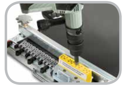
Electric Powered Rivet Driver Installation
