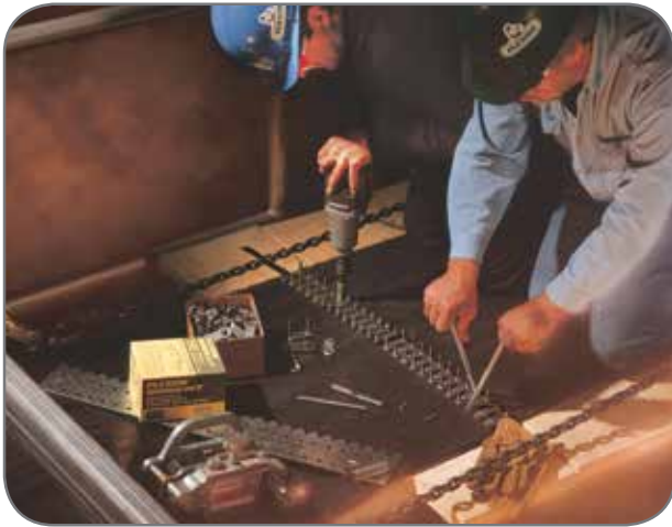
Mechanical fasteners can be installed by a variety of on-site, easy-to-use tools.
