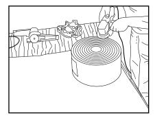
**2.** Use a grinding wheel (or variable speed buffer with a buffing disc) to buff the edges and bottom of the lagging.
