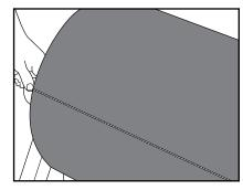
5. After the first coat of adhesive has dried completely, mark a line across the pulley face, parallel to the shaft's centerline and square to the edge of the pulley.
