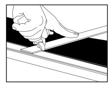
**3.** Use the strip selection chart (at the bottom of the page) to calculate the number of strips required for your pulley diameter. Lagging strips should be cut 4 inches (100 mm) longer than the pulley face width. **Note:** Do not allow ceramic tiles to sit at, or over, the edge of the pulley face.
