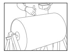
1. Prepare the pulley by removing the old lagging, paint, and primer. Sand blast the entire pulley (or use a grinding wheel) including the edges, and paint the pulley surface, including the edges, with metal primer recommended by the adhesive manufacturer. Allow to dry completely – follow adhesive manufacturer's recommendation.
