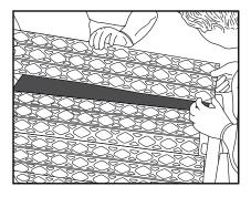
12. Follow steps 6 through 10 to install remaining pieces. The final piece of lagging (the largest of the final pieces) should drop into position. You may want to check the fit of the last piece prior to applying the second coat of adhesive.
