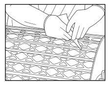
**13**. Seal any gaps between the lagging strips with rubber sealer.
