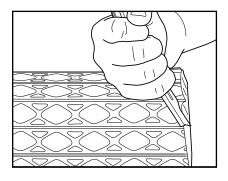
10. Trim the excess lagging from applied strips at the edge of the pulley. Trim lagging at an angle up and away from the pulley edge. Coat cut edge and joint area between lagging strips.
