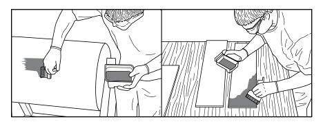
**4.** After mixing the adhesive according to the manufacturer's instructions, immediately apply the first coat to the entire pulley surface and all strips of lagging.
