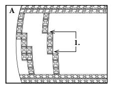
11(A). To lag the remainder of the pulley, position cut off pieces of lagging from step 10 and position in the unlagged portion of the pulley. Manipulate pieces to determine trim requirements (1.) Trim pieces at gutters as required for proper fit
