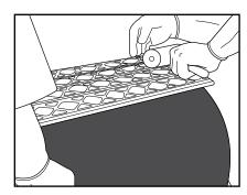
8. After the second coat has reached the appropriate tackiness (follow adhesive manufacturer's recommendation) install one strip of lagging. Use the perpendicular line to assure that the strip is square to the pulley. Working out from the center of the strip, use a dead blow hammer or pneumatic sand rammer to remove air gaps. Repeat this process with a stitcher to remove air gaps from the drainage grooves.
