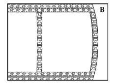
11(B). Test fit sample pieces at both edges and at pulley center to ensure optimal fit. Use trimmed test fit pieces as templates for trimming the final strips of lagging.
