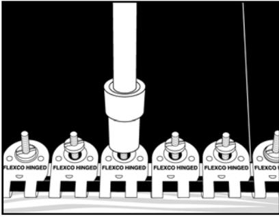
**NOTE:** Use Flexco Power Wrench (HW1) or Flexco Hand Wrench (S1S) when installing stainless steel or Everdur nuts.
