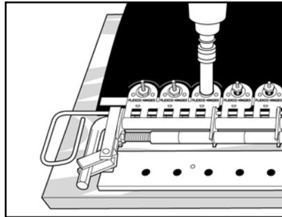
**14.** Tighten nuts in each 3-plate strip with wrench. The fastener teeth should penetrate the belt. Rubber covered belts should pucker around the top plates.
