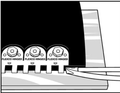
**19.** Insert filler tubing into fastener loops. Use gauge pin to guide the filler tubing into place. Pull out gauge pin.
