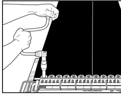
**11.** Tighten both end nuts using Flexco Hand Wrench (100) in a ½" (12mm) square hole ratchet or carpenter's brace.
