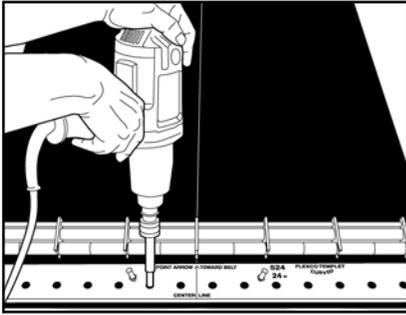
5. Punch holes using Flexco Punch. For quicker installation use the Flexco Power Punch with an impact tool.
