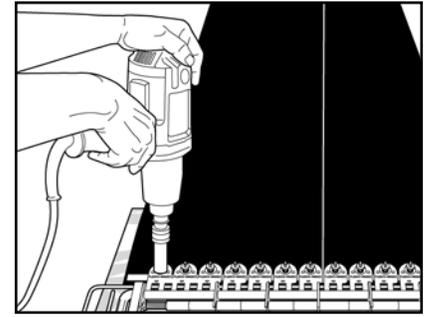
**12.** For quicker installation use a Flexco Power Wrench (H100) and impact tool.
