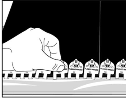
6. Remove aligning holder. If using 3-plate strips, place strips at splice ends. Insert fasteners and tighten nuts by hand. Slots in bolt heads must be engaged with lugs on fasteners.
