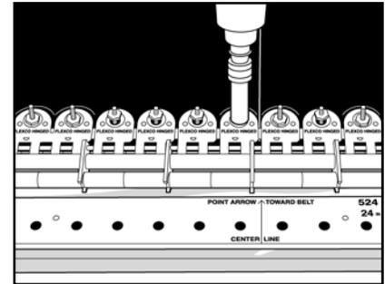
**15.** Tighten center nut then remaining nuts with wrench. The fastener teeth should penetrate the belt. Rubber covered belts should pucker around the top plates.
