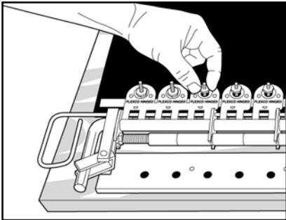
**13.** Skip steps 13 and 14 if not using 3-plate strips. Tighten by hand the remaining two nuts in each 3-plate strip as tight as possible. The slots in the bolts must engage the lugs on fasteners.
