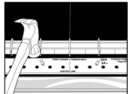
**4.** Nail aligning holder to belt. Bend nails at right angles to prevent shifting.
