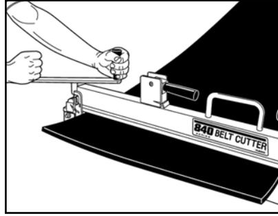
**1b.** For belt widths greater than 72" (1800mm), square belt and use Flexco 840 Series Belt Cutter to make a straight cut.
