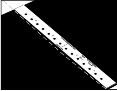
**1a.** For belt widths 72" (1800mm) or less, use Alligator® 400 Series Curved Belt Cutter to make a concave cut.
