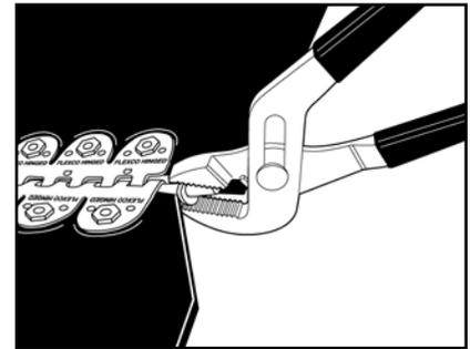
**21.** Notch trailing edge of belts 24" (600mm) and wider. Insert washer on hinge pin and crimp with pliers.
