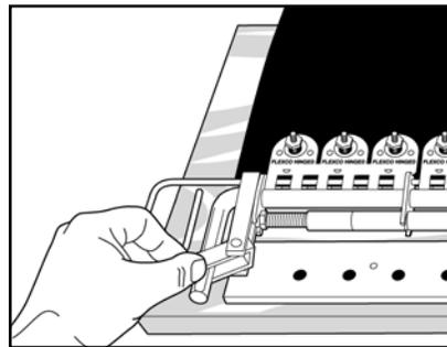
9. Insert gauge pin. Turn cam pin to horizontal position and lock with cam pin lock.
