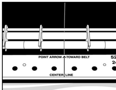
**3.** Place aligning holder on belt. Align the belt's centerline with the centerline on the aligning holder.
