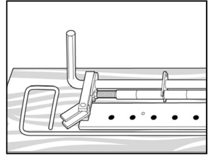
7. Remove gauge pin. Turn cam pin to upright position.
