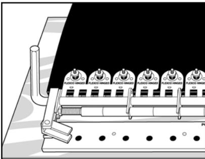
8. Starting at one end of the tool mesh aligning holder with fasteners.
