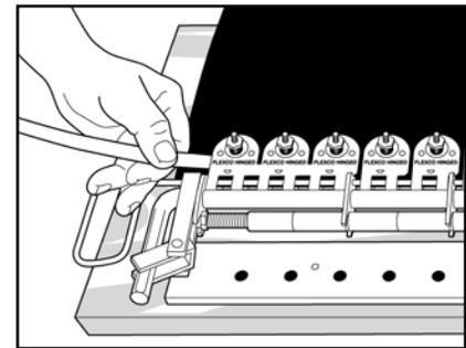
10. Cut two strips of Flexco-Lok® Tape the width of the belt. Feed one strip under top plates and one strip under bottom plates.
