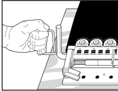
**17.** Move cam pin to the upright position. Remove gauge pin. Remove aligning holder from belt.
