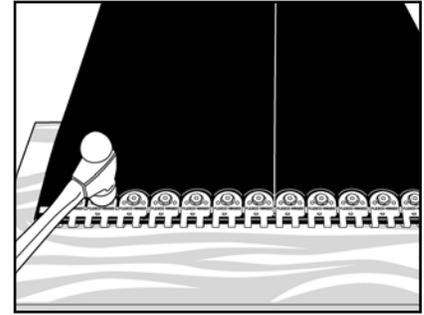
**18.** Peen or grind bolts to finish.
