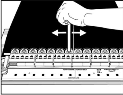
**16.** Break off excess bolt ends using Flexco Bolt Breaker. Use a slight rocking motion and keep the bolt breaker tight on the nut.
