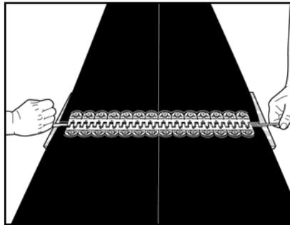
**20.** Repeat steps 1-19 on other belt end. Join belt ends. Insert gauge pin. Feed hinge pin from opposite side of the splice while backing out gauge pin.
