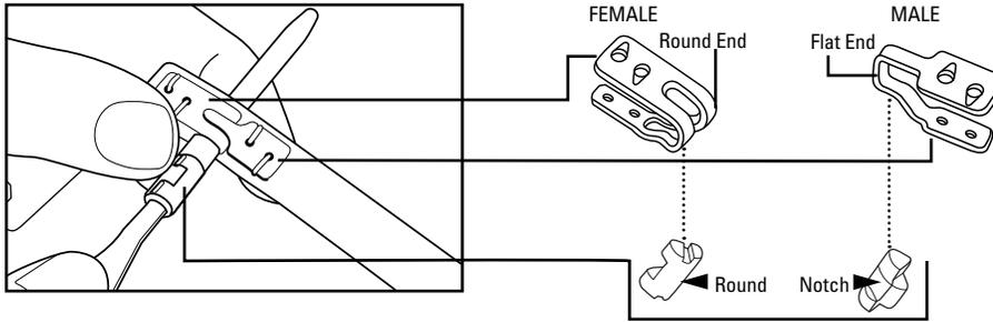
6. To make belt endless, mesh end-plates.
