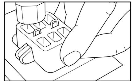
3. Push male or female half of fastener over belt and into recess in holder as far as it will go. Look into staple slot in holder and make sure holes in fastener are visible. Drive staple into belt flush with holder.
