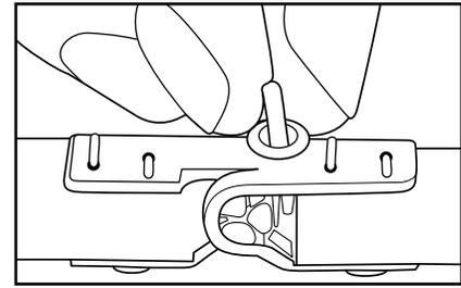
7. To keep rocker pins in place, push pin retainer through gap in top of fastener as shown.
