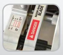
The FSK<sup>\*\*</sup> is offered with your choice of metal or plastic fence for adjusting the skive width. The metal fence is ideal for environments where consistent, repeat skive width is important.
