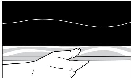
1. Place a wood support under belt where rip is to be repaired. Do not install Turtle® fasteners using the conveyor pulley or other metal surface as support, as fastener teeth would not be properly cinched.
