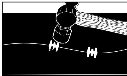
3. Drive fastener teeth into the belt and supporting board with a hammer. Avoid hitting the center of the plate.
