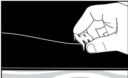
2. While holding ripped edges together place plates 4-6° apart with the fastener straddling both sides of the rip. A Turtle fastener may also be used at the end of a rip to prevent continued tearing.
