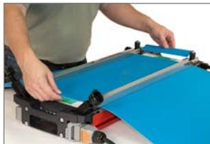
If bumpers are not abutted to the belt edges, melted material from the splice will flow off the belt ends, thinning out the spliced edges. This results in decreased strength in the fingers and overall splice.
