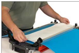
When the bumpers aren't filled to the width, including beyond the clamp bolts, even pressure is not attained. Uneven pressure causes uneven cooking, which may potentially cause inconsistent splices and air bubbles and pockets.
