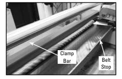
2. (Belt End 1) With the edge of the bottom cover against the c-clamp tray belt stop, fold top cover back clamping it between the clamp bar.
