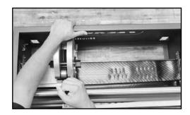
**10.** Begin punching the top cover by following instructions starting on pg.19 of the PUN M<sup>™</sup> Manual Finger Punch Safety and Operation Manual until you've utilized the complete cutting surface of the punch board.
