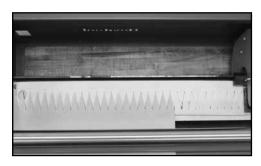
**15.** Prior to re-clamping and resuming punch process, measure the distance between the leading belt edge and the c-clamp tray stop on the left, and be sure the distance measures the same on the right leading belt edge prior to clamping and resuming punch process. Repeat process until the entire belt end has been punched.
