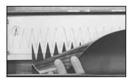
7. Prior to punching the top cover, release the clamp bar allowing the top cover to lay over the already punched fingers. Line up the left edge of the top cover with the peak on the left side of the punch board making sure the front edge of the top cover is up against the c-clamp tray belt stop and lock in place. Slide and lock the PUN M™ tray in the back position and resume the punch process until you've utilized the complete cutting surface of the punch board.
